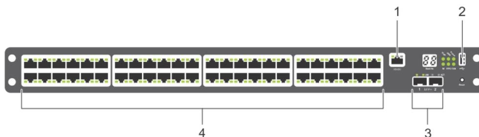
**Figure 1. N2048 Series with 48 10/100/1000BASE-T Ports**
