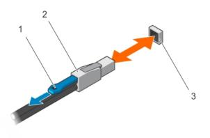
Figure 1. Connecting a SAS cable
