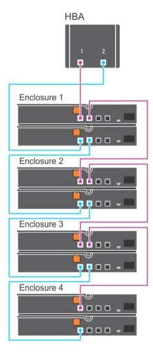
Figure 3. Redundant configuration
