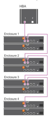
Figure 2. Single port configuration
