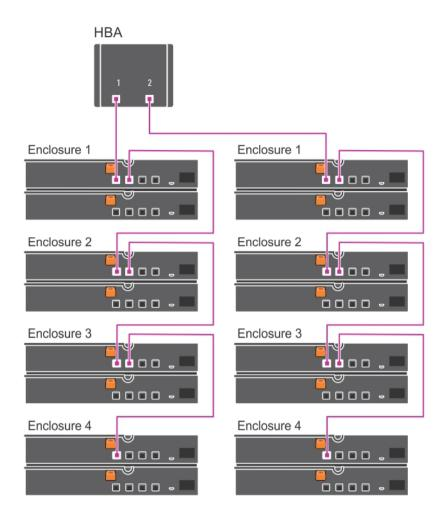
Figure 4. Multi-chain configuration
