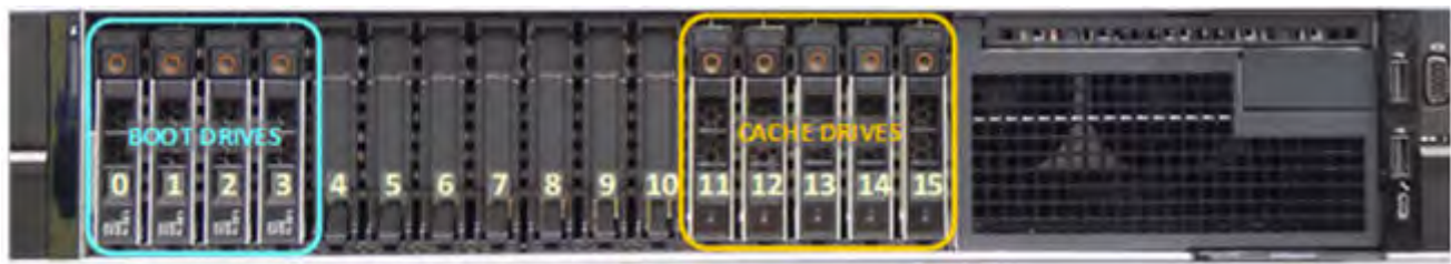
Figure 120. DD9400 SSD slot assignment (single node configuration)
