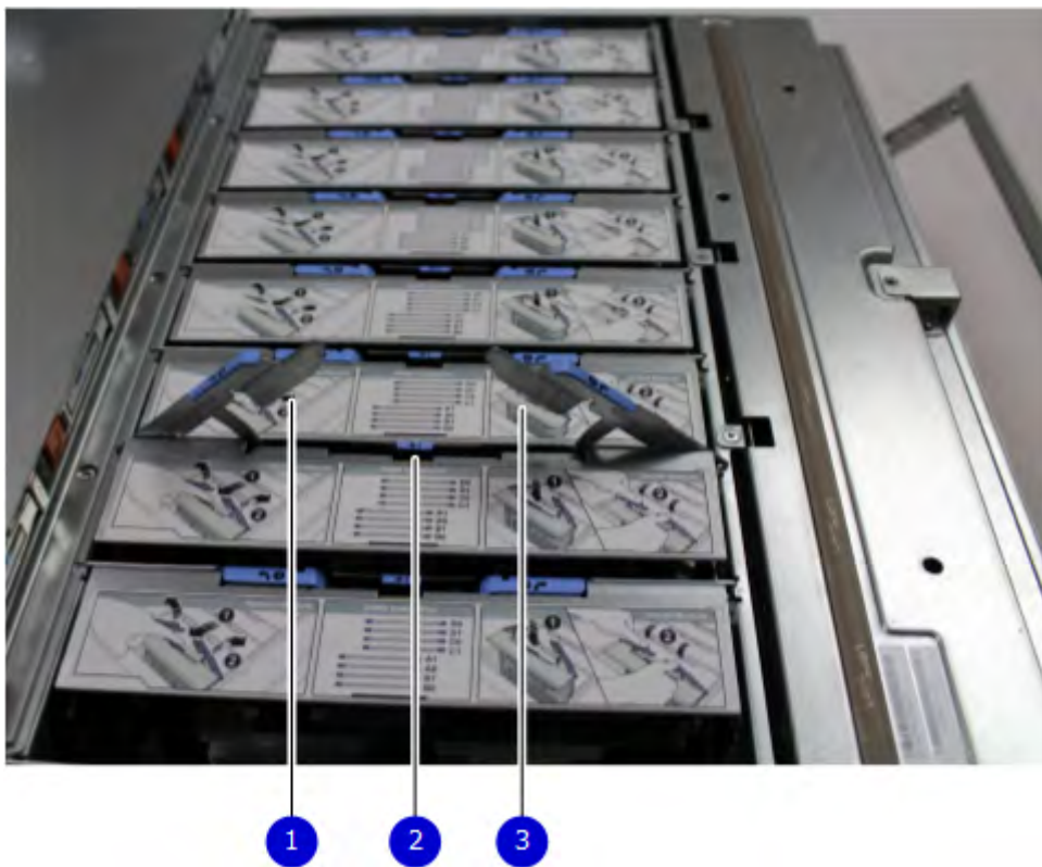
Figure 138. Releasing a memory riser
