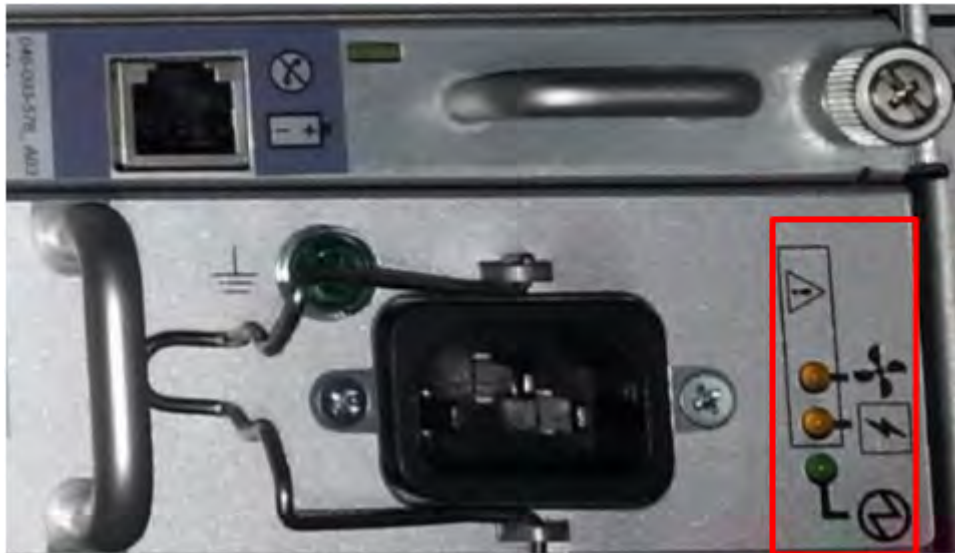
Figure 172. Power Supply A LEDs
