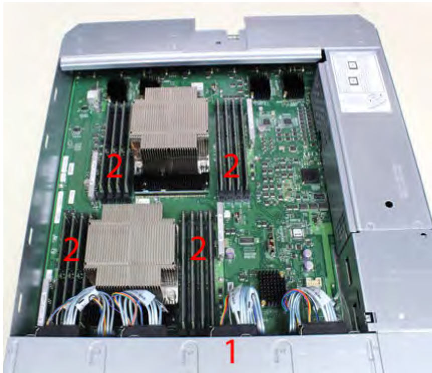
Figure 93. Top view of SP module with SP cover removed
