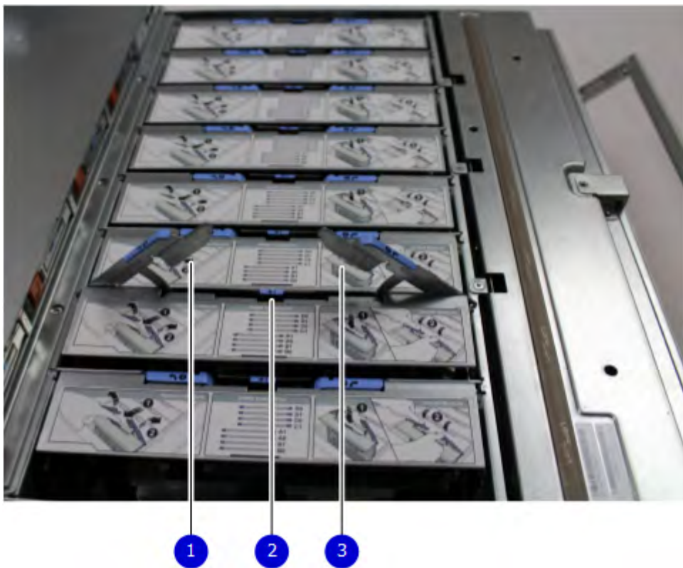
Figure 154. Releasing a memory riser
