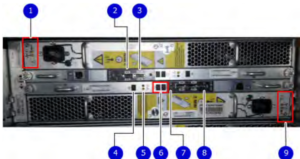
Figure 175. Back panel: Power modules and controllers
