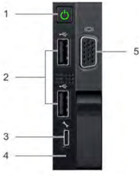
Figure 118. Front right control panel power button LEDs
