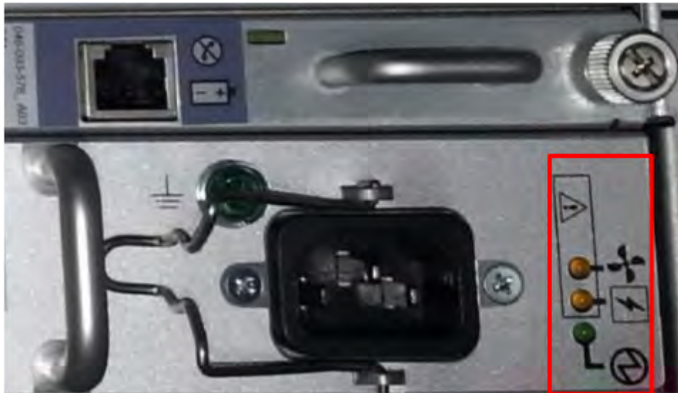
Figure 176. Power Supply A LEDs
