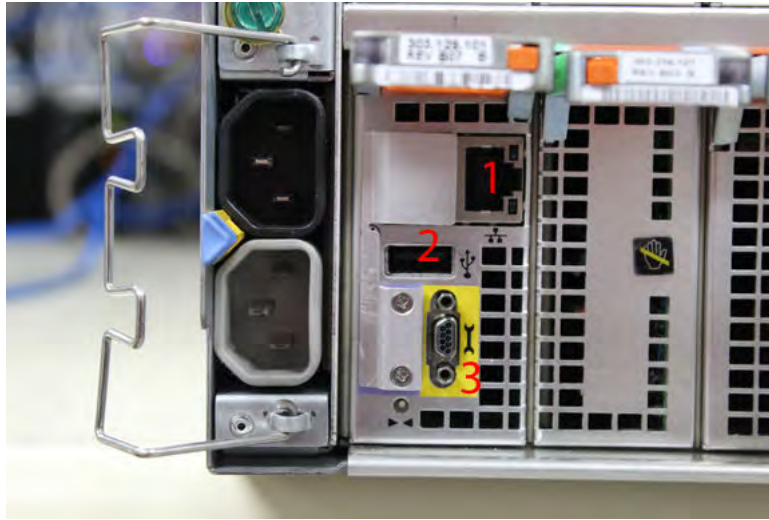
Figure 48. Interfaces on the management module
