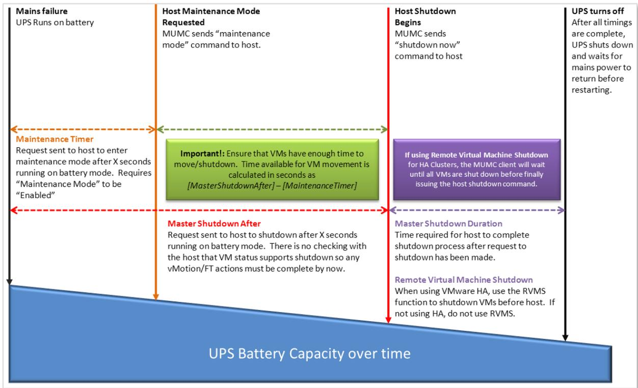
Figure 16: Shutdown sequence (from ULNM UG)
