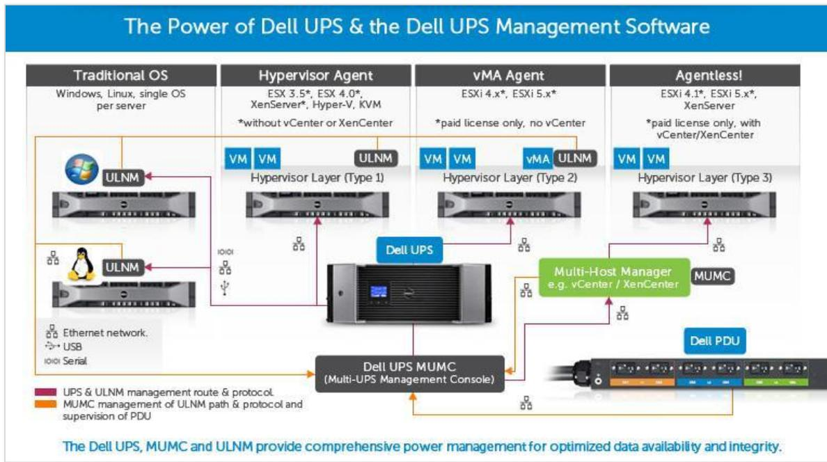
Figure 4: UPS management architecture in a virtualized environment
