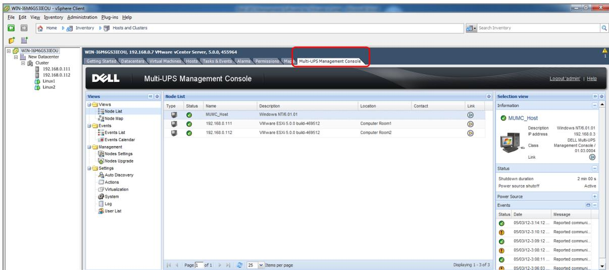
11. Within the MUMC client (vCenter plugin), navigate to Views → Node List and verify that all hypervisors are recognized.
