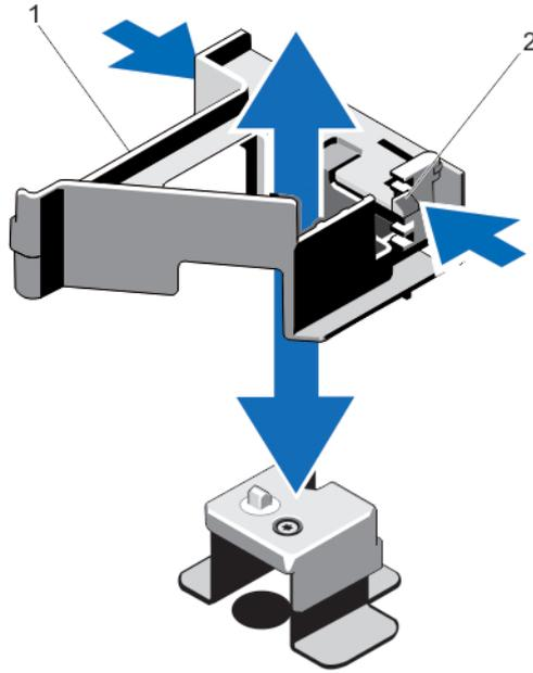
**Figure 19. Removing and Installing the PCIe Card Holder**
