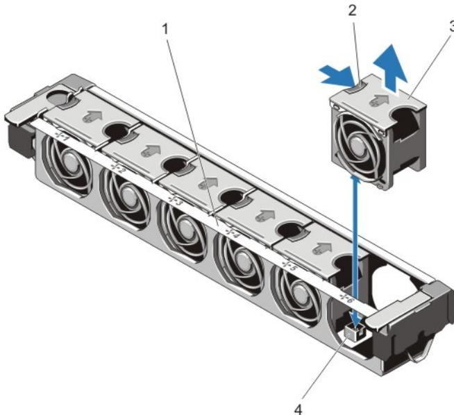
**Figure 16. Removing and Installing a Cooling Fan**
