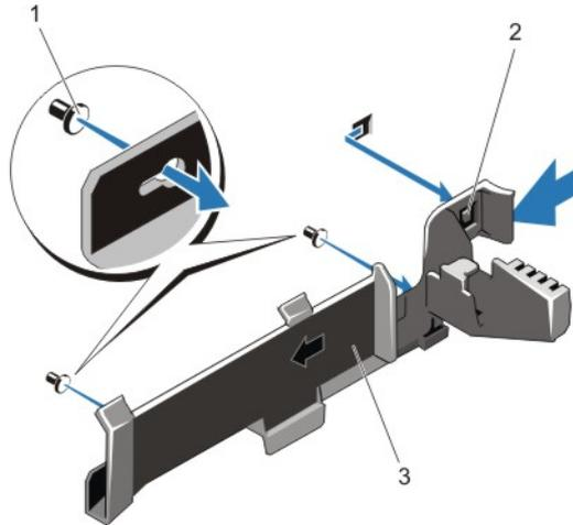
**Figure 21. Removing and Installing the Cable Retention Bracket**
