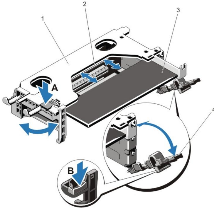
**Figure 23. Removing and Installing the Expansion-Card Riser 1**
