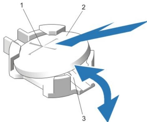
**Figure 43. Replacing the System Battery**
