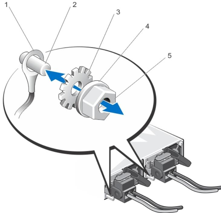
**Figure 39. Assembling and Connecting the Safety Ground Wire**
