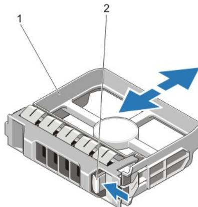
**Figure 14. Removing and Installing a 3.5 Inch Hard-Drive Blank**
