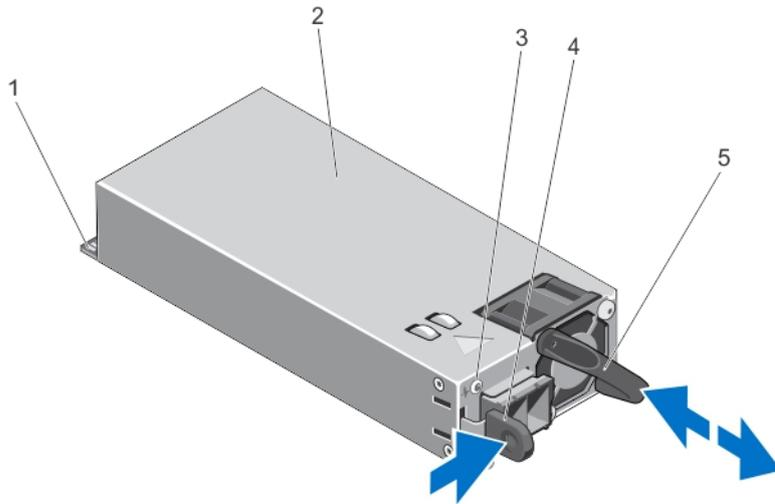
**Figure 41. Removing and Installing a DC Power Supply**
