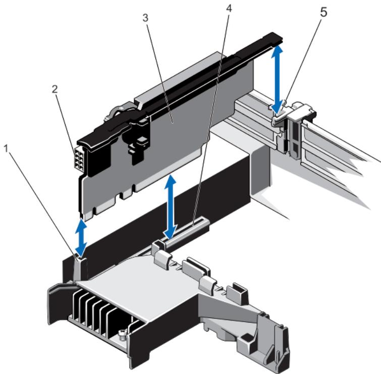
**Figure 28. Removing and Installing the Expansion Card Riser 3**
