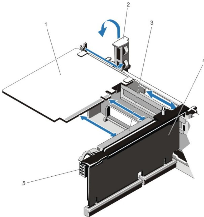
**Figure 22. Removing and Installing the Expansion Card**
