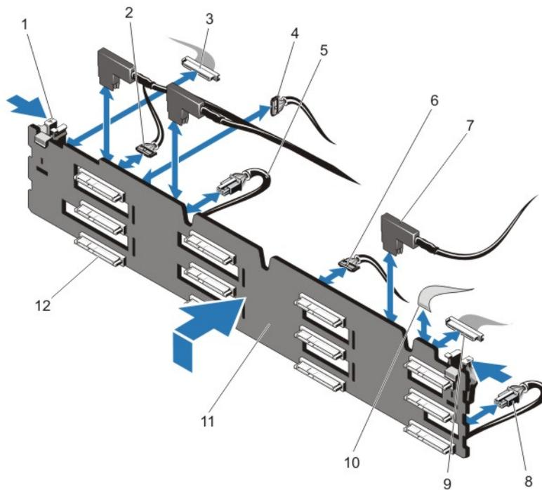
**Figure 44. Removing and Installing the 3.5 Inch (x12) SAS/SATA Backplane**
