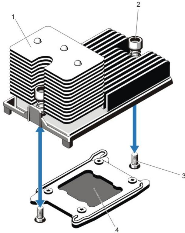
**Figure 35. Removing and Installing the Processor Heat Sink**
