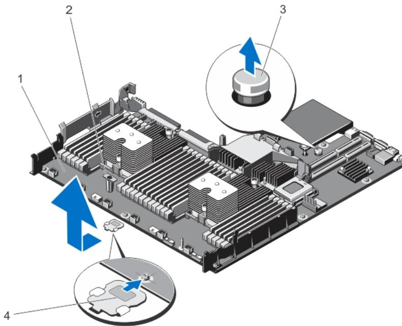
**Figure 50. Removing and Installing the System Board**
