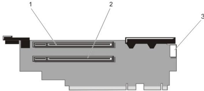
**Figure 29. Identifying Connectors on the Expansion Card Riser 3**
