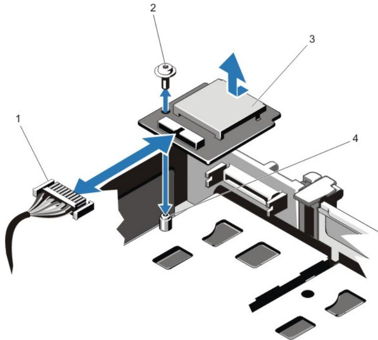
**Figure 31. Removing and Installing the vFlash Media Unit**
