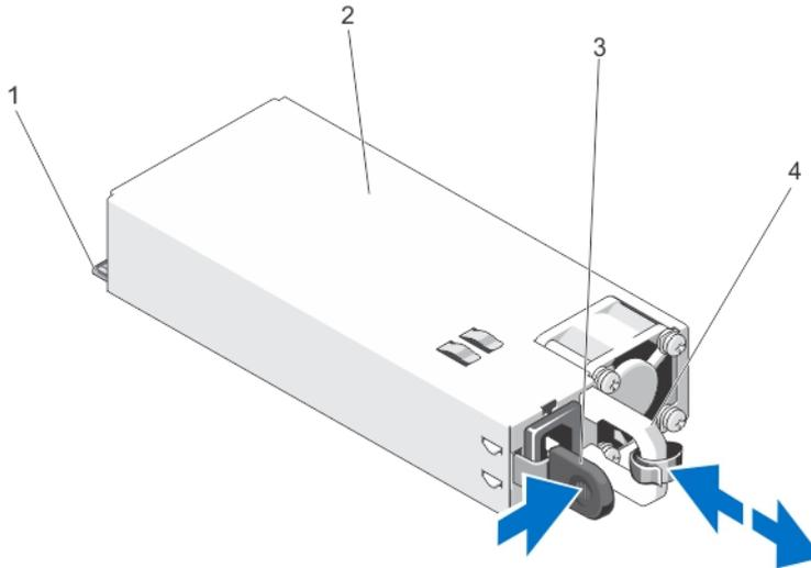
**Figure 38. Removing and Installing an AC Power Supply**
