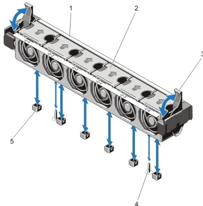
**Figure 17. Removing and Installing the Cooling-Fan Assembly**
