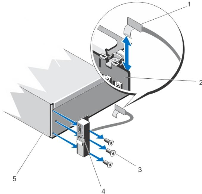
**Figure 49. Removing and Installing the I/O Panel**
