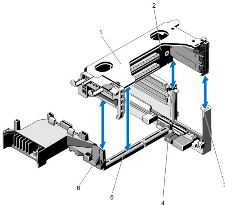
**Figure 24. Removing and Installing the Expansion Card Riser 1**
