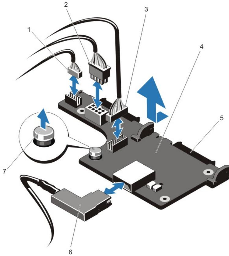
**Figure 46. Removing and Installing the Optional 2.5 Inch (x2) Hard-Drive Backplane (back)**
