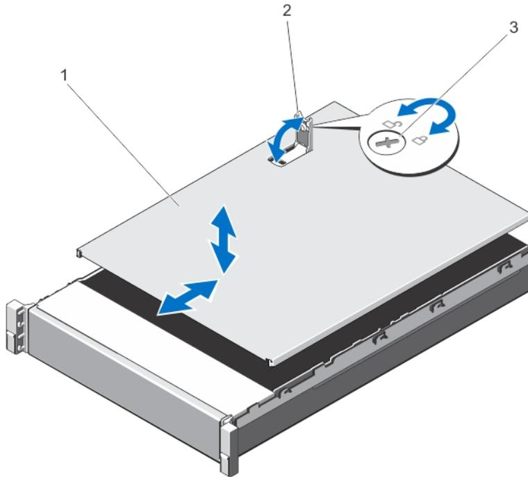
**Figure 8. Opening and Closing the System**
