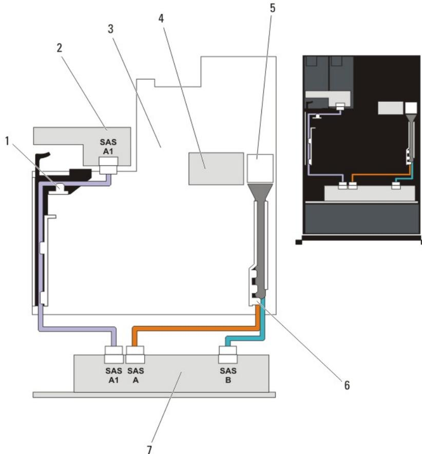
**Figure 47. Cabling Diagram—Optional 2.5 Inch (x2) Hard-Drive Backplane (back)**
