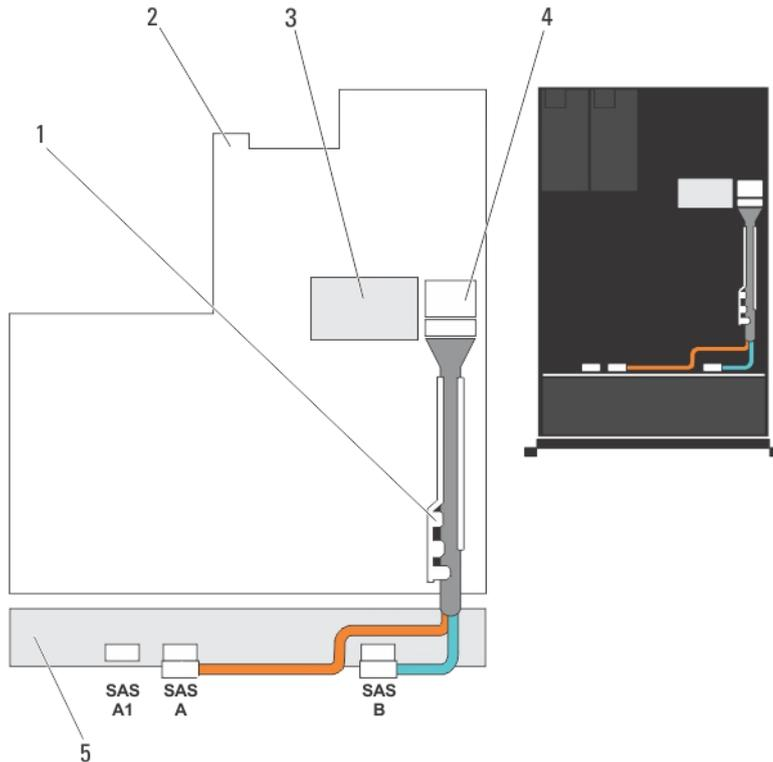
**Figure 45. Cabling Diagram—3.5 inch (x12) SAS/SATA Backplane**
