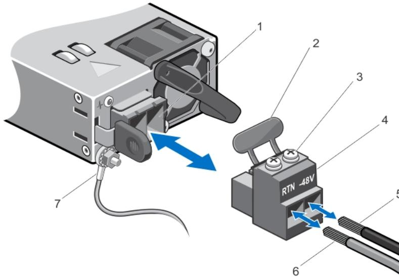
**Figure 40. Assembling the DC Input Power Wires**
