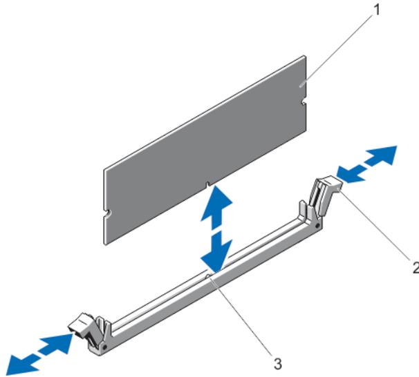
**Figure 12. Removing and Installing a Memory Module**
