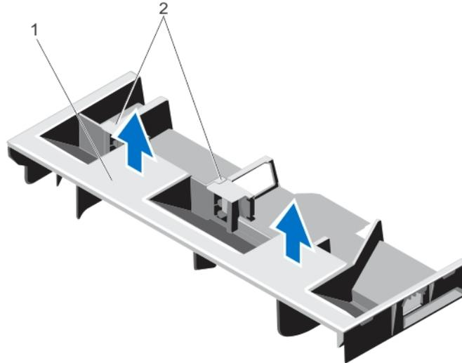
**Figure 10. Removing and Installing the Cooling Shroud**
