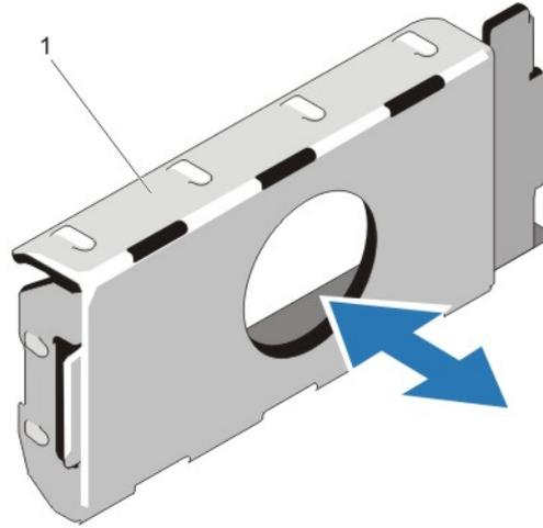
Figure 42. Removing and Installing the Power Supply Blank
