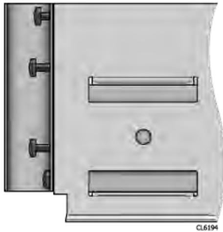
2. Attach a short bracket to the rear of each rail using two M5 screws into the top and bottom holes.
