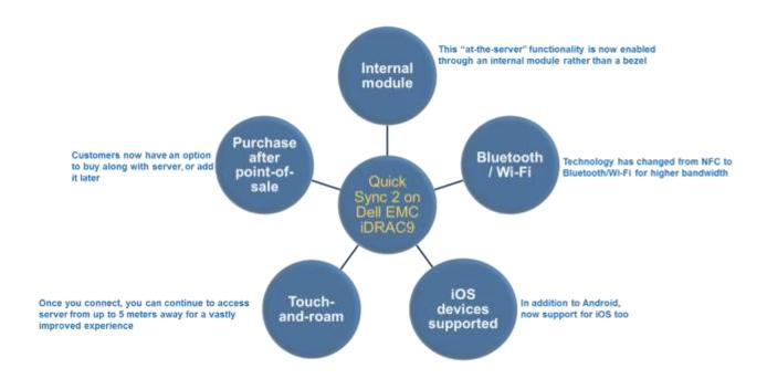
Quick Sync 2 is supported on all 14G rack and most tower servers. Please contact Sales for latest information on Quick Sync 2 support for any specific 14G server. Quick Sync 2 extends our lead in at-the-server systems management which already includes iDRAC Direct that enables customers to access server through a notebook PC or easily configure it with an SCP file (Server Configuration Profile) stored on a USB drive.
