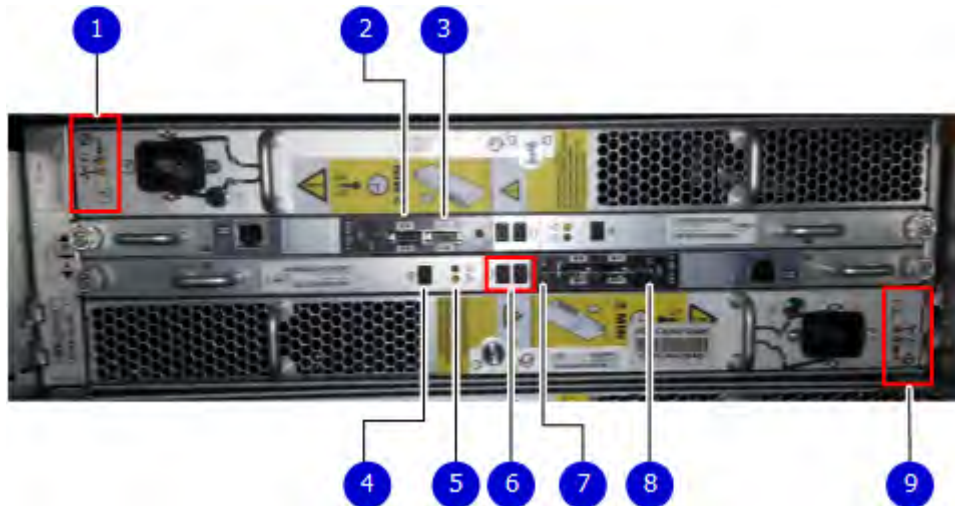
Figure 181. Back panel: Power modules and controllers
