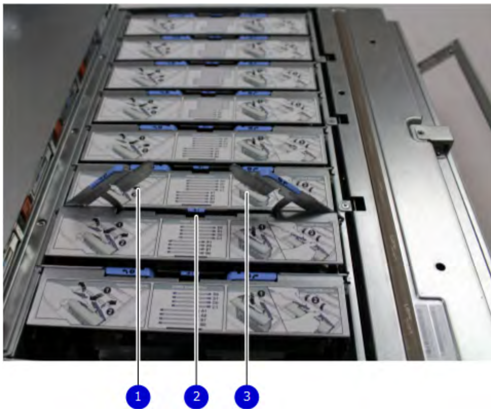
Figure 172. Releasing a memory riser
