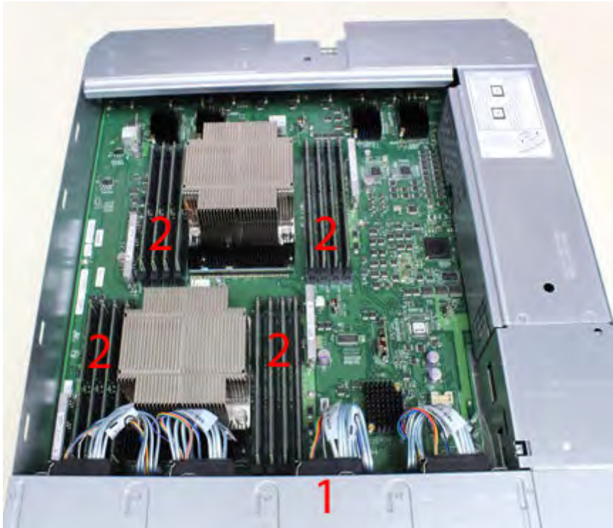
Figure 107. Top view of SP module with SP cover removed
