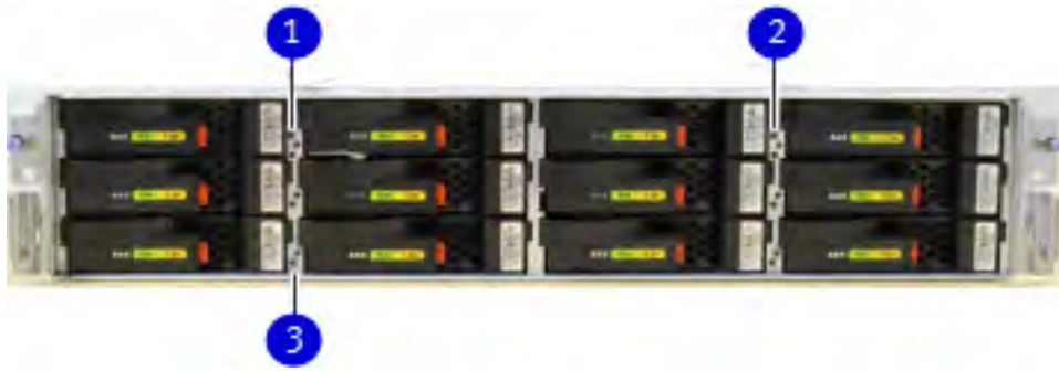
Figure 73. Disk and system LEDs
