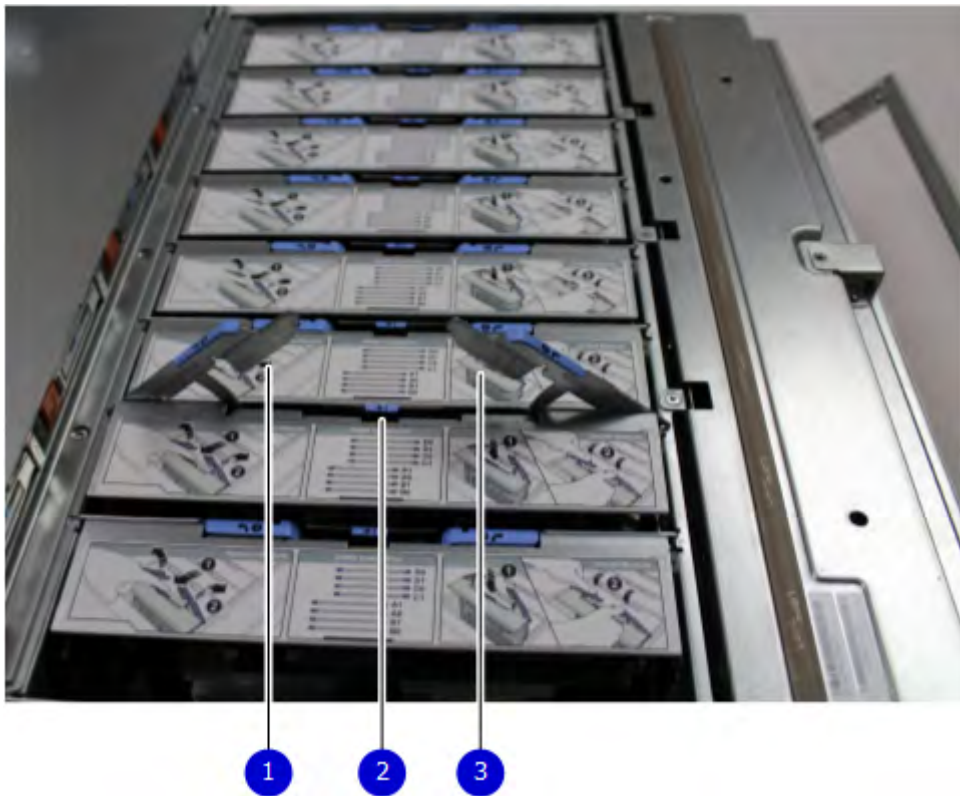
Figure 156. Releasing a memory riser
