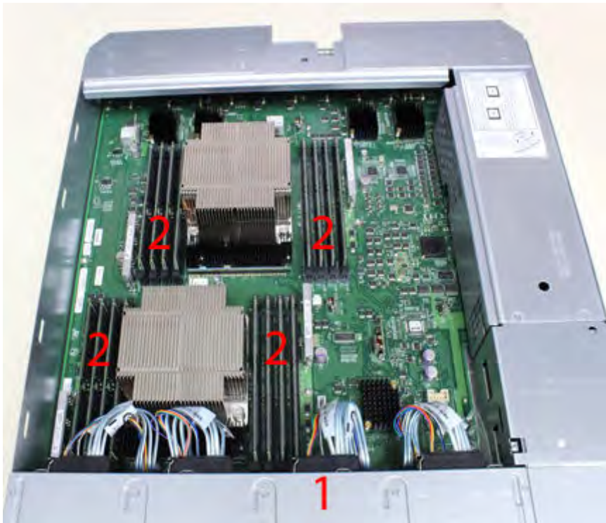
Figure 115. Top view of SP module with SP cover removed
