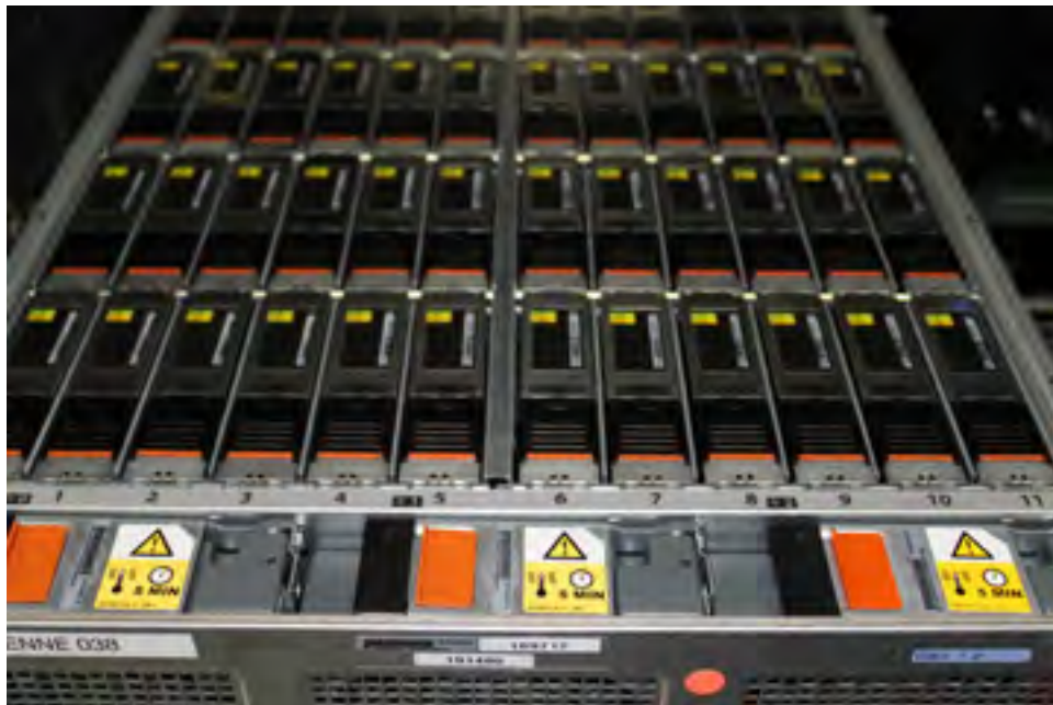
Figure 176. Fans and disk drives inside the disk enclosure
