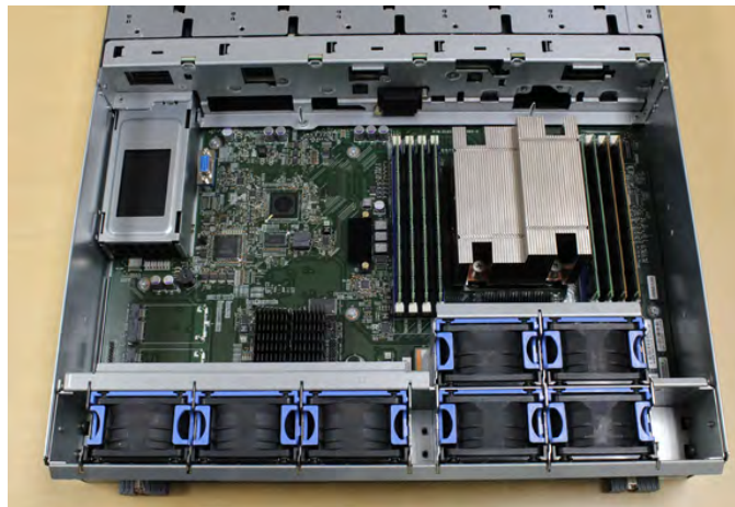
Figure 79. Top view of SP module with air ducts removed
