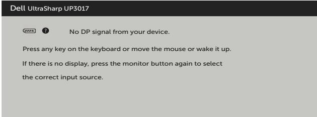
If either DP, mDP, HDMI1 or HDMI2 input is selected and the corresponding cable is not connected, a floating dialog box as shown below appears.
