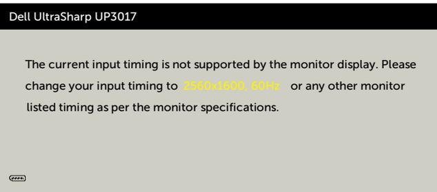
This means that the monitor cannot synchronize with the signal that it is receiving from the computer. See [Monitor Specifications](#) for the Horizontal and Vertical frequency ranges addressable by this monitor. Recommended mode is 2560 x 1600.
