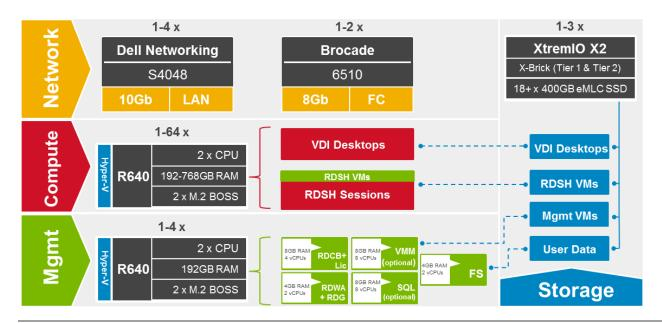
**NOTE**: Minimum disk configuration per XtremIO X2 X-Brick is 18 x 400GB SSDs which is sufficient for up to 3500 VDI users. Additional disks may be required if increased capacity is needed for larger personal disk sizes and if user data is also stored on the array.
