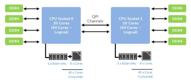
To ensure no NUMA spanning, remove the checkmark for "Allow virtual machines to span physical NUMA nodes" in the Hyper-V settings of the compute host(s). Also ensure "Maximum NUMA nodes allowed on a socket" is set to a value of 1. This setting is found under Processor > NUMA for each RDSH VM.
