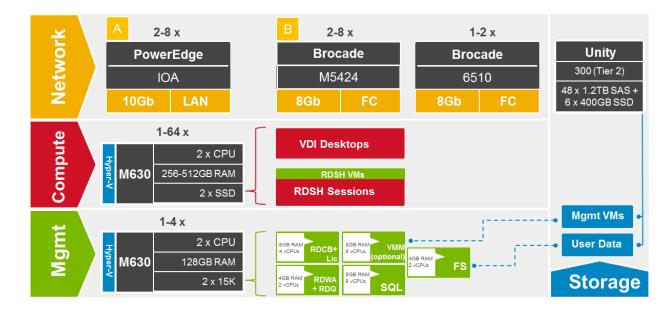
Note: This configuration only possible by installing OS and virtual machines on same set of disks and RAID controller which may impact performance. Compute disk size depends on total capacity requirements.
