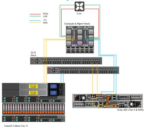
Refer to the Unity 300 Tier 2 section for a diagram of disk enclosure connections via mini-SAS HD.
