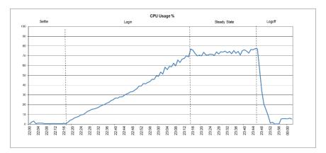
450GB of memory was used during the test stay within the 90% threshold limit. Although CPU usage and IO latency are low, the system is limited by available memory.
