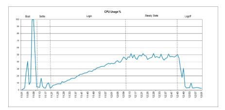
450GB of memory was used during the test to stay within the 90% threshold limit. Although CPU usage and IO latency are low, the system is limited by the memory available.
