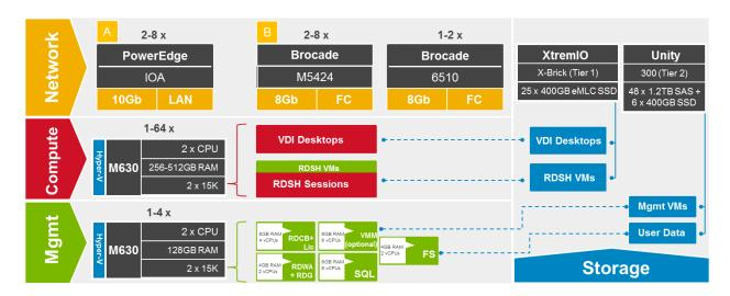
Note: Maximum of 64 nodes supported per cluster, but each cluster limited to a maximum of 8000 running virtual machines.
