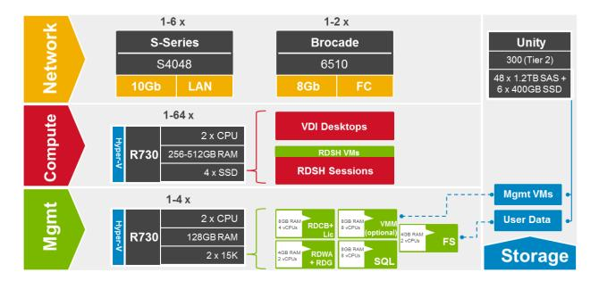
Note: Compute disk size depends on total capacity requirements. Recommended minimum of 4 x 800GB SSDs.
