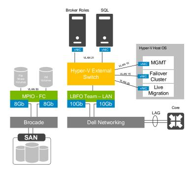
The dedicated compute host configuration is shown in the diagram below and configured similarly to the management host configuration but without the features enabled by shared storage.
