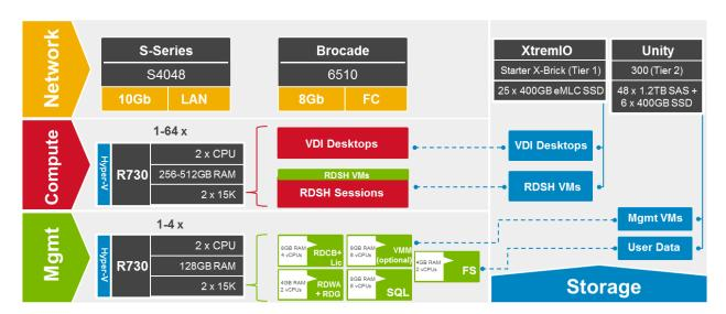
Note: Maximum of 64 nodes supported per cluster, but each cluster limited to a maximum of 8000 running virtual machines.
