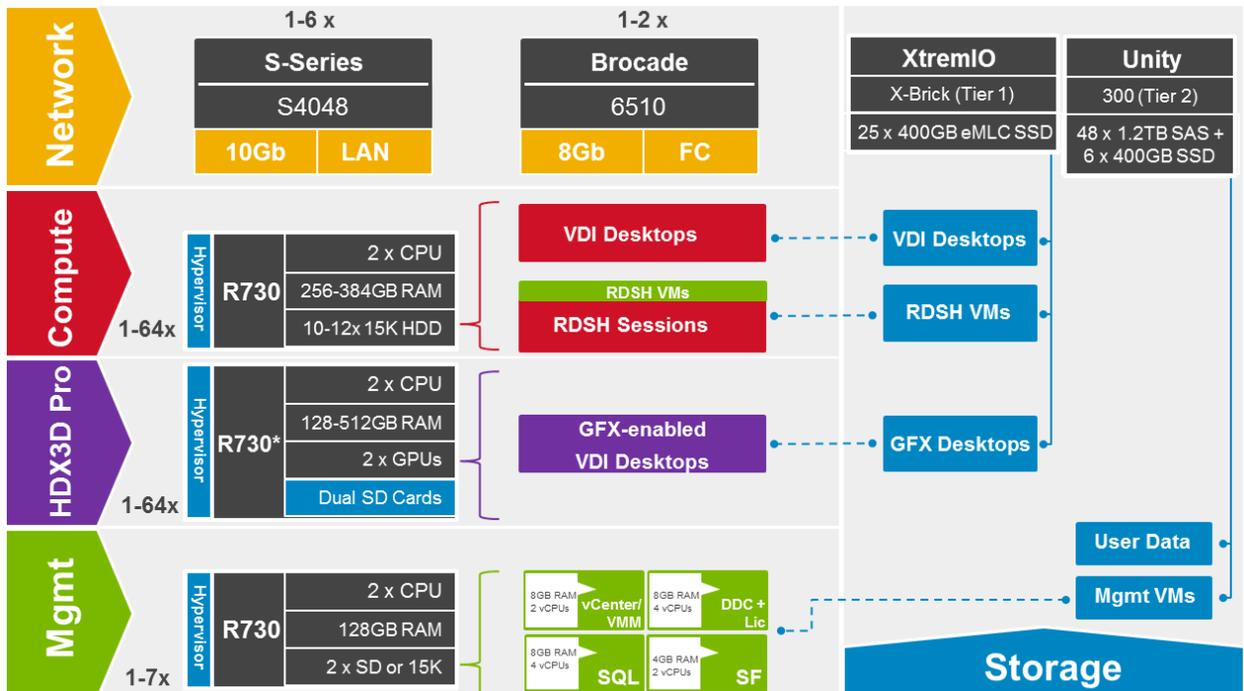
\* The Dell Precision Appliance for Wyse is a R730 server based solution
