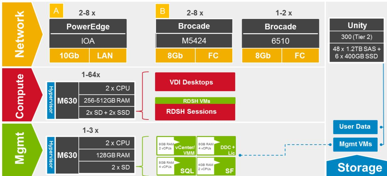
**Note:** Hypervisor installation to SD cards is recommended for vSphere but not supported for Hyper-V.
