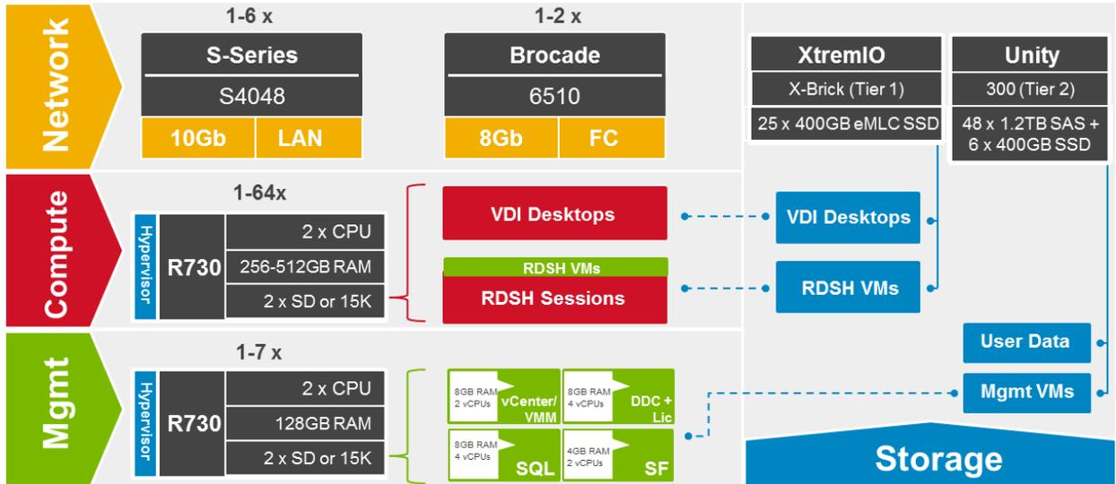
The diagram below shows the discrete T1 and T2 arrays with a graphics-enabled compute configuration.
