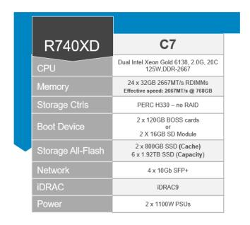
This configuration would be classed as an AF-8 (All-Flash) on the vSRN HCL.
