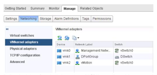
The distributed switch configuration is the same on all VSRN storage hosts. It is recommended to have at least two uplinks for each host to provide load balancing and fail back redundancy.
