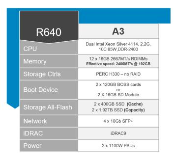
This configuration would be classed as an AF-4 (All-Flash) on the vSRN HCL.
