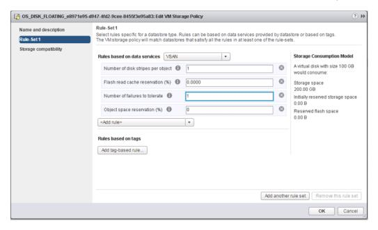
The recommended configuration by VMware for a vSAN Cluster with FTT=1 and Raid 1 is four nodes and this ensures that the virtual machines are fully protected during operational & maintenance activities. This configuration can also survive another failure even when there is a host already in maintenance mode.
