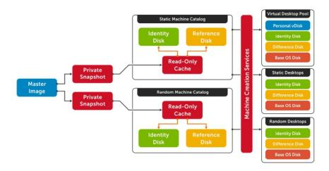
While traditionally used for small to medium sized XenDesktop deployments, MCS can bring along with it some substantial Tier 1 storage cost savings because of the snapshot/identity/difference disk methodology. The Tier 1 disk space requirements of the identity and difference disks when layered on top of a master image snapshot, is far less than that of a dedicated desktop architecture.
