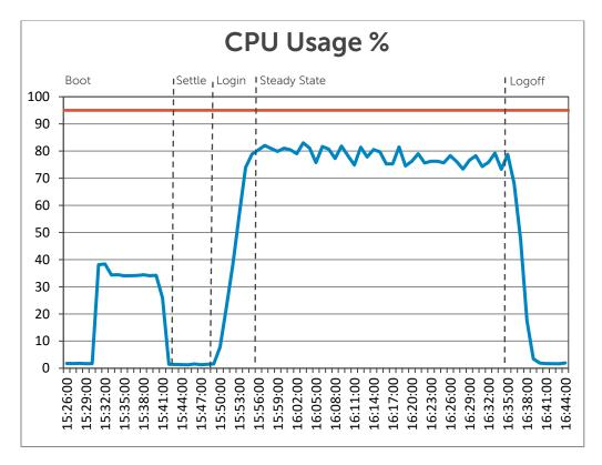
CPU usage for 32 clients is averaging below the 95% acceptance mark for this particular CPU [with Turbo enabled]. Maximum possible clients for the profile M60-1Q with a 2 GPU board/server configuration is 32 clients with a maximum resolution of 4096x2160. Maximum resolution was not used in this test since the test environment does presently not support this resolution. The resolution used was 1920x1080.
