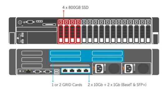
**NOTE:** The default disk configuration is shown in the diagram here; however, this can be modified to match the customer's local storage needs.
