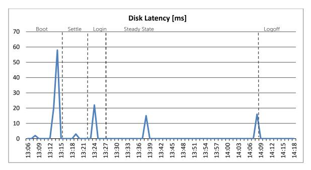
Highest disk activity was observed during the boot period. Tests were configured in such a way as to launch a session on a Client VM in 10 second intervals. After all clients have launched, processing values settle for the steady state values.
