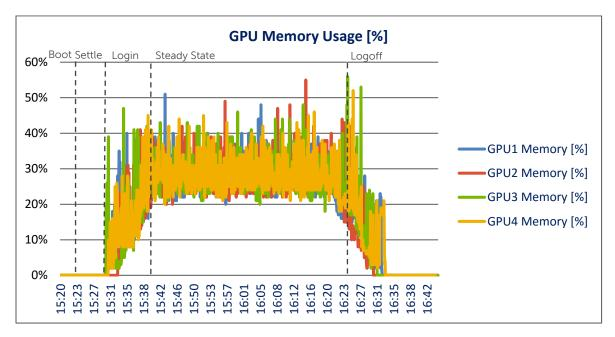
On average 28% GPU memory was used during steady state testing. GPU memory utilization will depend on the graphics applications itself. High GPU memory usage should not be expected with the workload.
