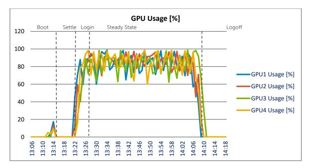
During steady-state average GPU processor utilization shows 84%. GPUs are expected to run at full capacity. A low GPU load could point to issues with server CPUs not being able to handle the graphics load or other issues holding back the GPU. This is not the case here.
