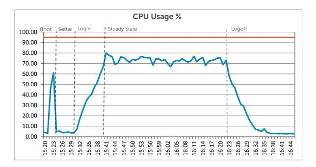
CPU usage for 64 clients is averaging 73% which is below the 95% threshold.
