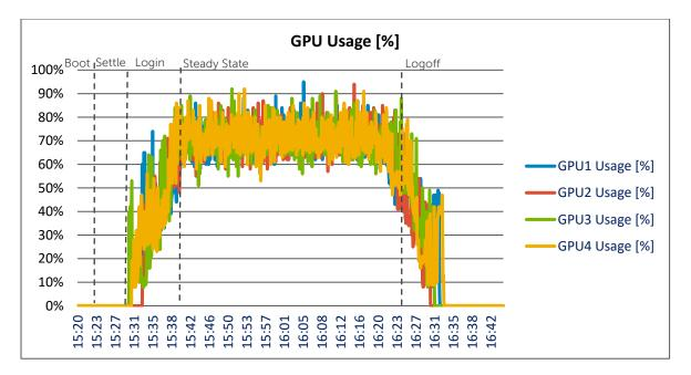
During steady-state average GPU processor utilization shows 70%. GPUs are expected to run at full capacity. A low GPU load could point to issues with server CPUs not being able to handle the graphics load or other issues holding back the GPU. This is not the case here.
