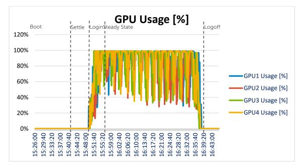
During steady-state average GPU processor utilization shows 87%. GPUs are expected to run at full capacity. A low GPU load could point to issues with server CPUs not being able to handle the graphics load or other issues holding back the GPU. This is not the case here.
