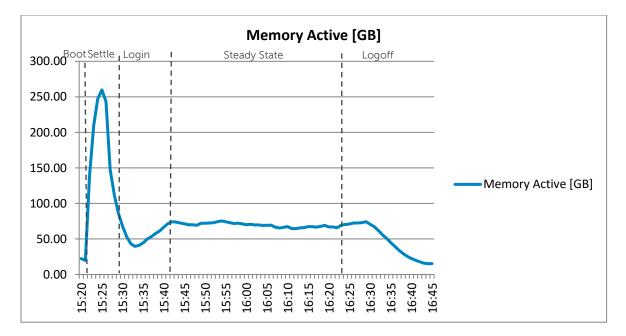
Host memory shows no bottle neck. For 64 clients with 4GB reserved RAM consumed memory should be 256GB + an overhead for vSphere services. On average the memory actively used by the clients is around half of the available memory. Swap Used [GB] and Balloon [GB] show 0 GB throughout the test.
