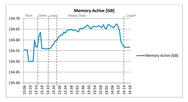
Host memory shows no bottle neck. For 32 clients with 4GB reserved RAM consumed memory should be 128GB + an overhead for vSphere services. On average the memory actively used by the clients is around half of the available memory. Swap Used [GB] and Balloon [GB] show 0 GB throughout the test.
