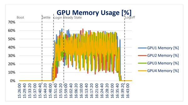
On average 39% GPU memory was used during steady state testing. GPU memory utilization will depend on the graphics applications itself. SPECview module sw-03 could be considered a medium graphics load. High GPU memory usage should not be expected with this module.
