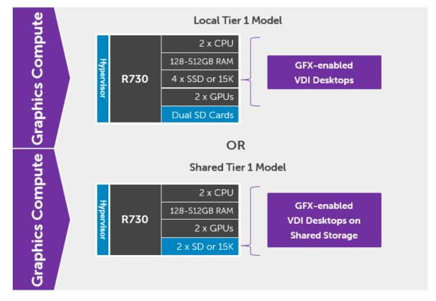
Designed to be compute nodes with graphics acceleration, the appliances fit in perfectly with the Local Tier 1 for Rack and Shared Tier 1 for Rack models of the Dell Wyse Datacenter solutions offerings. In the image
