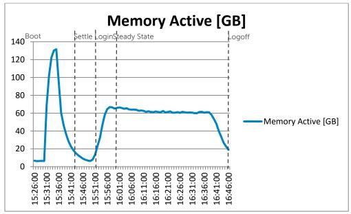
Host memory shows no bottle neck. For 32 clients with 4GB reserved RAM consumed memory should be 128GB + an overhead for vSphere services. On average the memory actively used by the clients is around half of the available memory. Swap Used [GB] and Balloon [GB] show 0 GB throughout the test.
