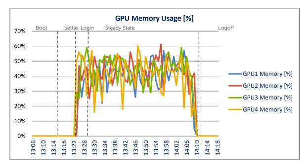
On average, 43% GPU memory was used during steady state testing. GPU memory utilization will depend on the graphics applications itself. SPECview module sw-03 could be considered a medium graphics load. High GPU memory usage should not be expected with this module.
