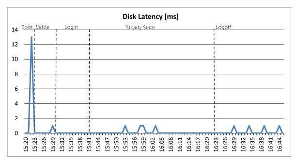
Highest disk activity was observed during the boot period. Tests were configured in such a way as to launch a session on a Client VM in 10 second intervals. After all clients have launched, processing values settle for the steady state values. Disk IOPS were observed to be still higher than the settled value at this point, completing the login process. During the indicated Steady State period, IOPS per user average 21. IOPS will eventually settle to a value of 15 IOPS per user.
