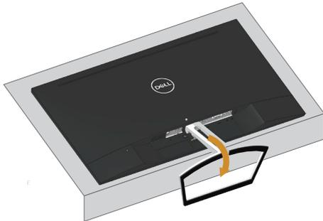
3. Use a long screwdriver to press on the release button.
