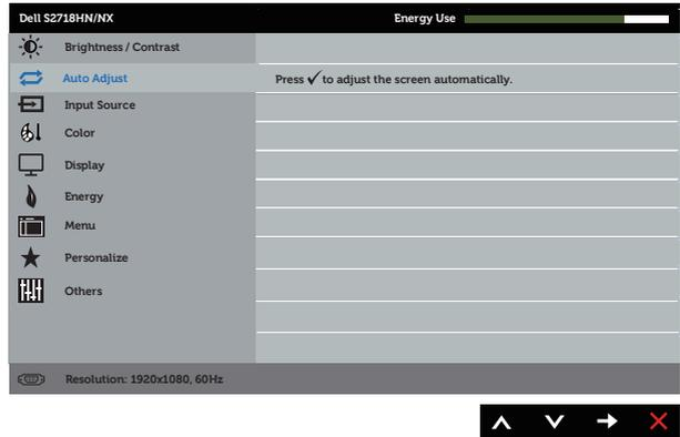
The following dialog appears on a black screen as the monitor self-adjusts to the current input:
