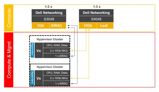
The following figure shows a design of a scale-out Leaf-Spine network architecture that provides 20 GB active throughput from each node to its Leaf and scalable 80 GB active throughput from each Leaf to Spine switch providing scale from 3 VxRail Appliance nodes to 64 without any impact to available bandwidth:
