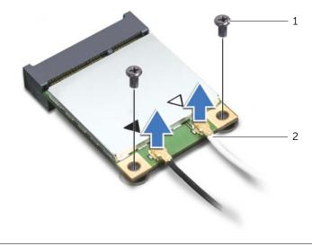
4 Slide and remove the wireless mini-card out of the wireless mini-card connector.
