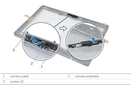
**3** Release the tabs that secure the camera module to the camera bracket and remove the camera module.
