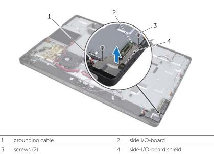
**3** Gently lift the side I/O-board starting from the inner edge and then ease the ports on the side I/O-board out of the slots on the display bezel.
