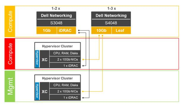
Designed for true linear scaling, XC Series leverages a Leaf-Spine network architecture. A Leaf-Spine architecture consists of two network tiers: a 10Gb layer-2 (L2) Leaf segment and a layer-3 (L3) Spine segment based on 40GbE and non-blocking switches. This architecture maintains consistent performance without any throughput reduction due to a static maximum of three hops from any node in the network.
