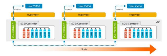
DSF virtualizes local storage from all appliances into a unified pool. DSF uses local SSDs and capacity disks from all appliances to store virtual machine data. Virtual machines running on the cluster write data to DSF as if they were writing to local storage. Nutanix data locality ensures that the XC Series node providing CPU and
