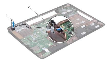
1 screw 2 AC-adapter connector cable
