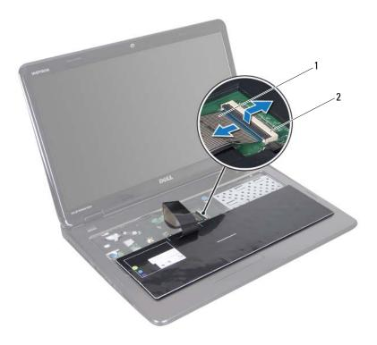
1 keyboard cable 2 keyboard-cable connector
