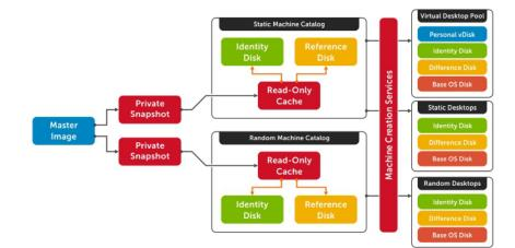
While traditionally used for small to medium sized XenDesktop deployments, MCS can bring along with it some substantial Tier 1 storage cost savings because of the snapshot/identity/difference disk
