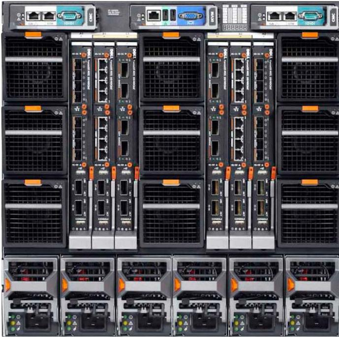
After you slide the MXL 10/40GbE Switch in so that the connectors on the back of the blade touch the chassis midplane, the switch receives power from the chassis and automatically powers on. The chassis management controller (CMC) in the chassis validates that the switch blade is a supported I/O module before powering it on.
