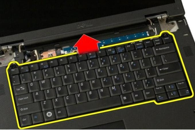
6. Open the keyboard data cable clip to free the ribbon cable.
