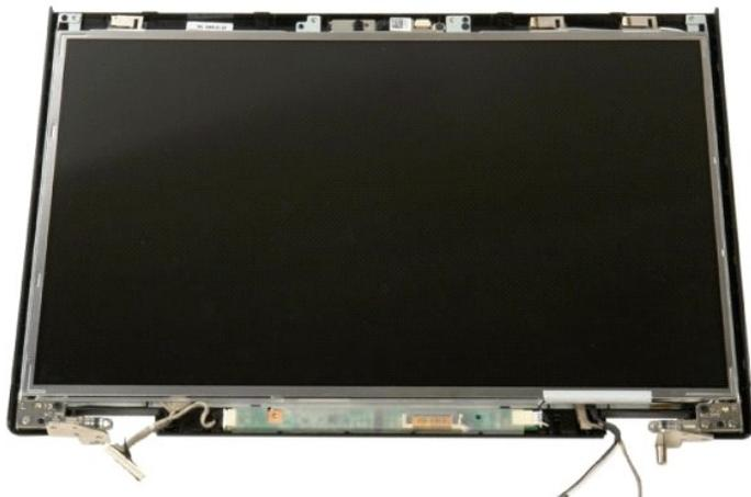
3. Remove the screw that secures the display inverter to the display assembly.
