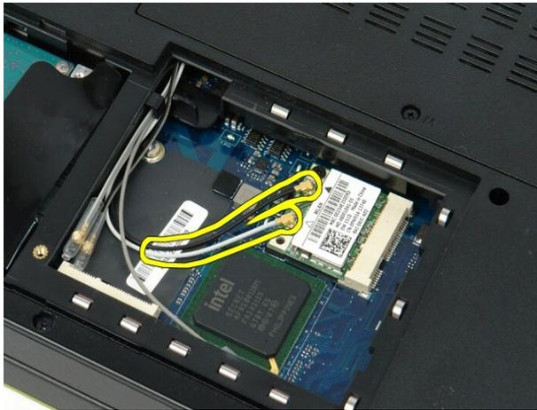
5. Remove the screw that secures the WLAN card to the system board.
