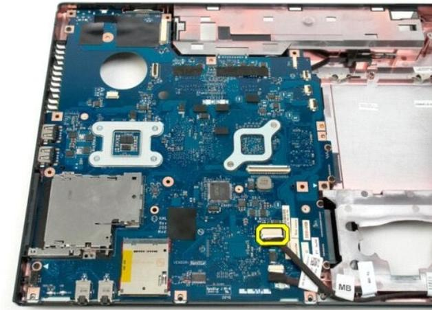
19. Disconnect the second data cable from the system board.
