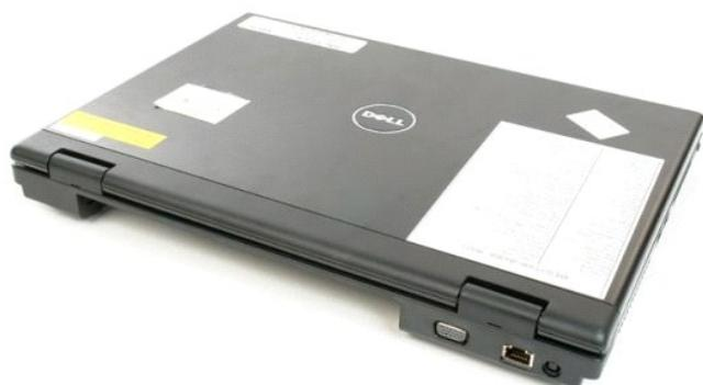
3. Use a plastic scribe gently to pry the back side of the hinge cover away from the base of the computer.
