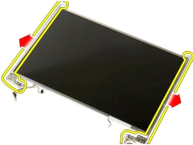
8. Remove the display panel hinges from the display panel assembly.
