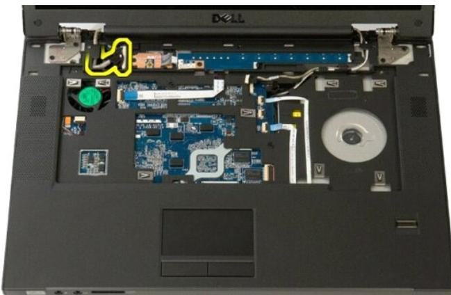
11. Carefully draw the antenna cables through the system board.
