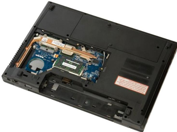
5. Loosen the six captive screws that secure the heat sink to the system board.
