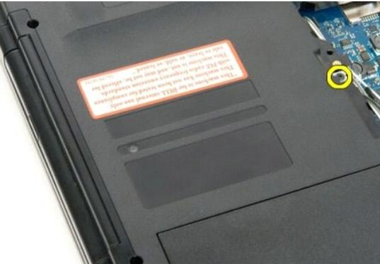
5. Insert a plastic scribe into the notch and slide the optical drive slightly out of the computer.
