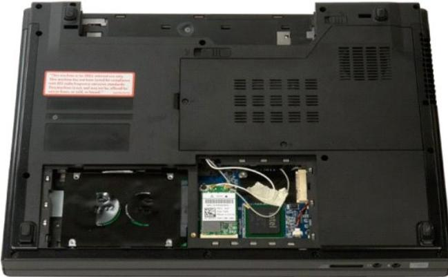
8. Disconnect the antenna cables from the WLAN card.
