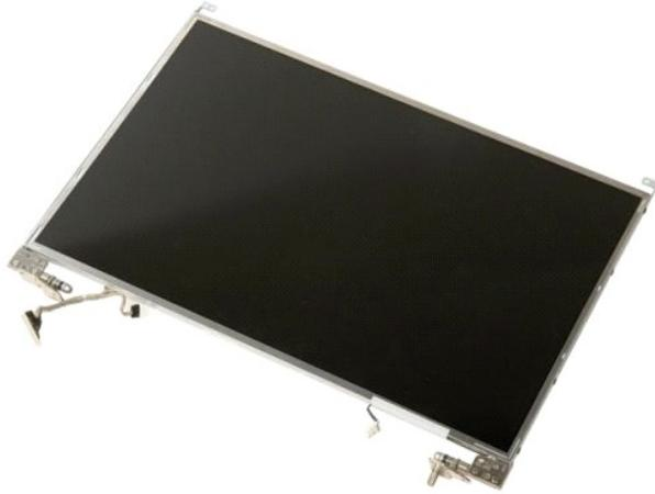
6. Remove the eight screws securing the hinges to the display panel assembly.
