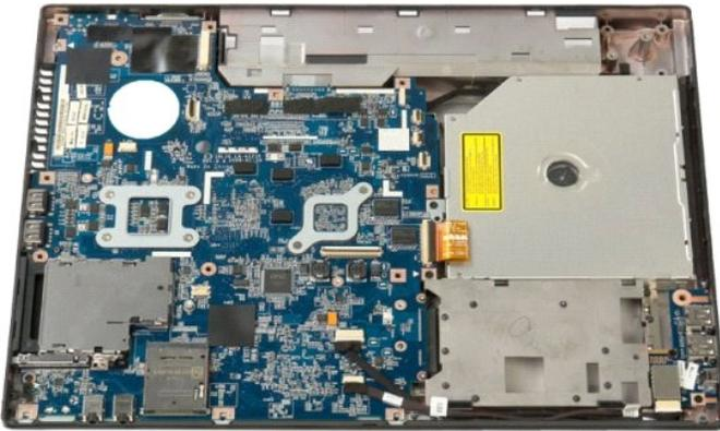
10. Remove the screw that secures the Bluetooth module to the system board.
